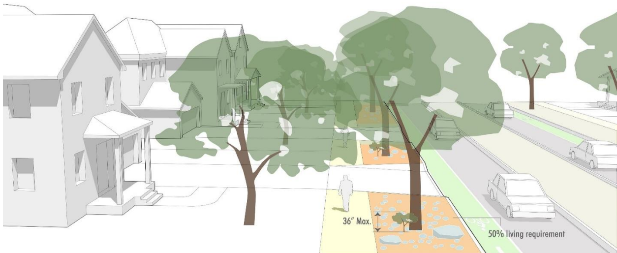
Figure 18.44-5b: Tree sidewalk clearance - residential
